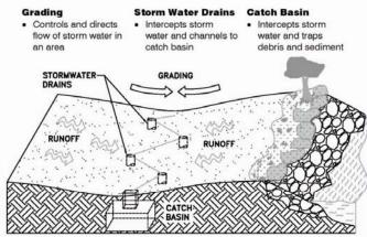
Storm water runoff can flush accumulated oils and pollutants from upland surfaces into nearby bodies of water. Pollution from multiple sources, known as non-point source pollution, can be managed through site planning that incorporates catchment, interception, and containment of run-off.
