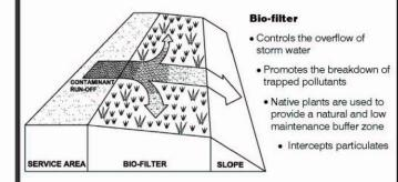
Bio-filtration helps remove contaminants potentially contained in water run-off.
