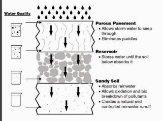
Rainwater runoff can flush accumulated pollutants from paved surfaces into nearby bodies of water. Porous paving filters these contaminants out and allows for bio-decomposition.
